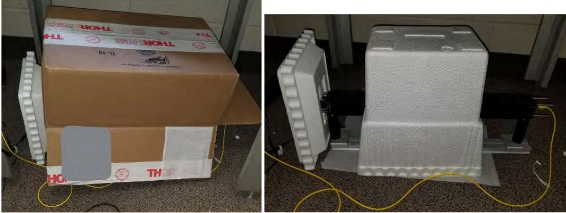
Figure 6. Images of the control experiment setup AIRFLOW covered by a cardboard box over the Styrofoam box (left) AIRFLOW’s sampling area covered in a Styrofoam box (right)
